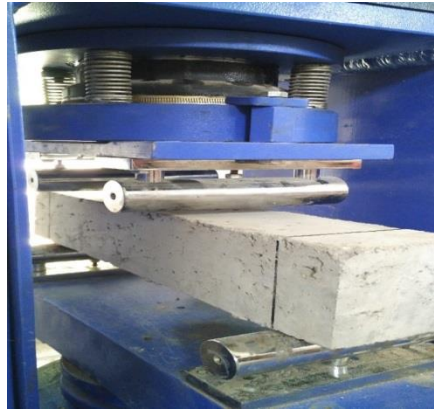
Figure.6. Setup for Flexure Strength Test
