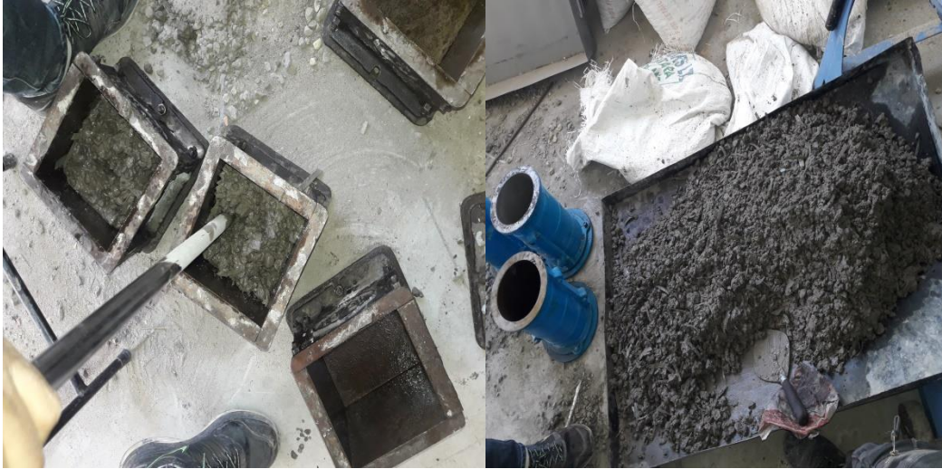
Figure.4. Casting of Specimens
